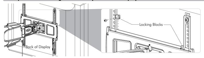
Step 7. Adjust Arm movement if necessary
