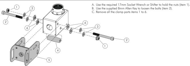
Step 3. Assemble the clamp parts to B2B Head Assembly
